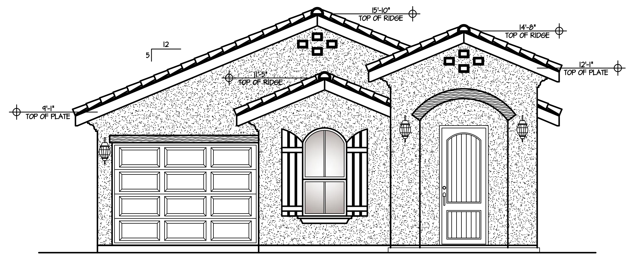
FRONT ELEVATION 'A' SCALE: 1/4" = 1'-0"
