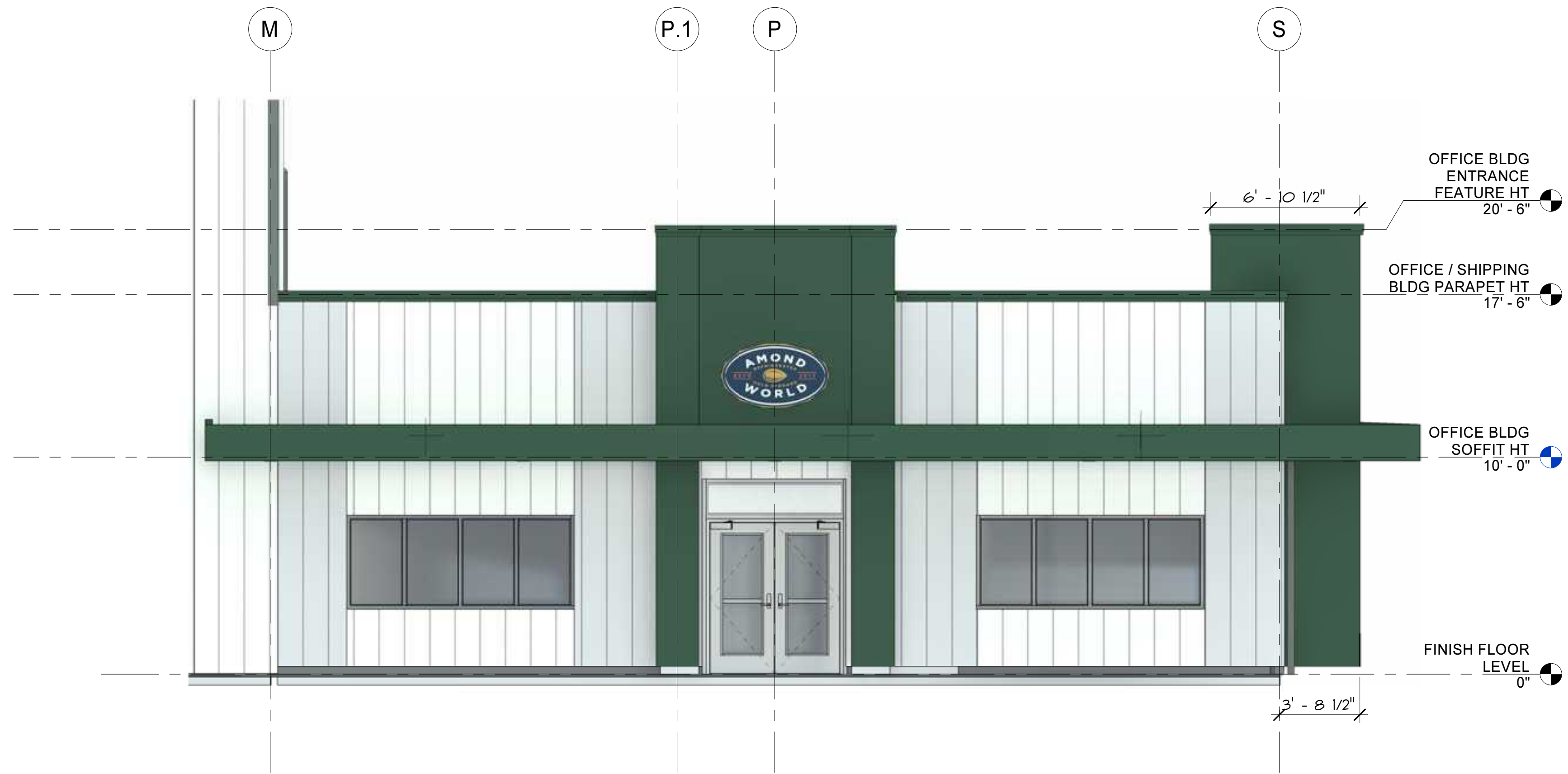
2 OFFICE BUILDING- ELEVATION 1 1/4" = 1'-0"
