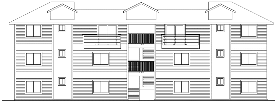
BUILDING E EAST ELEVATION
