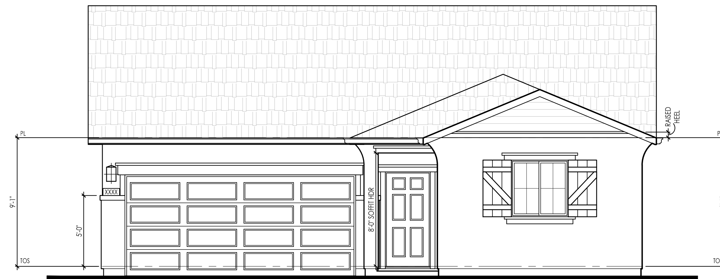
'COTTAGE' (COMPOSITION SHINGLE) FRONT ELEVATION "C"
