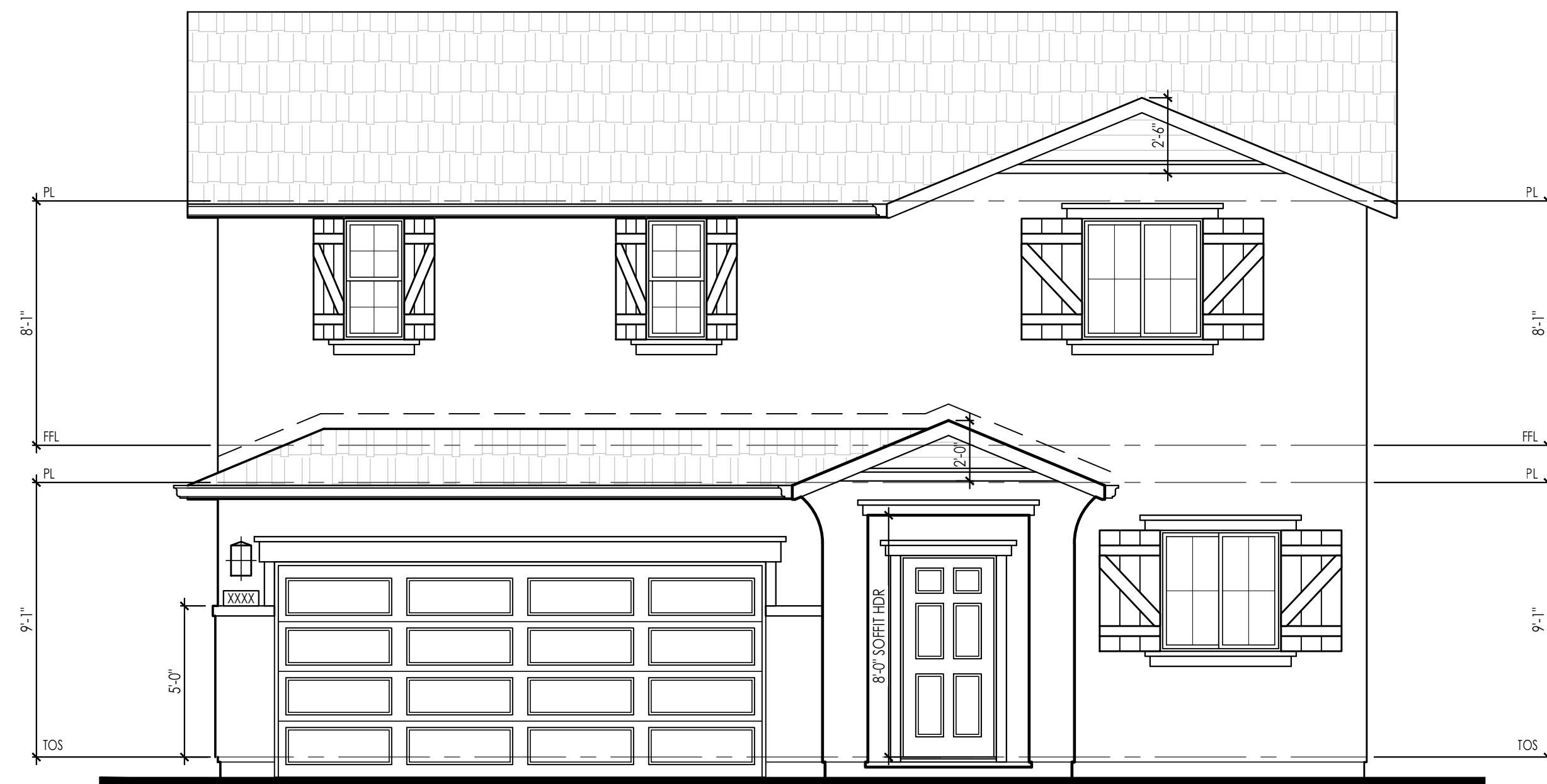
'COTTAGE' (COMPOSITION SHINGLE) FRONT ELEVATION "C" 1/4" = 1'-0"
