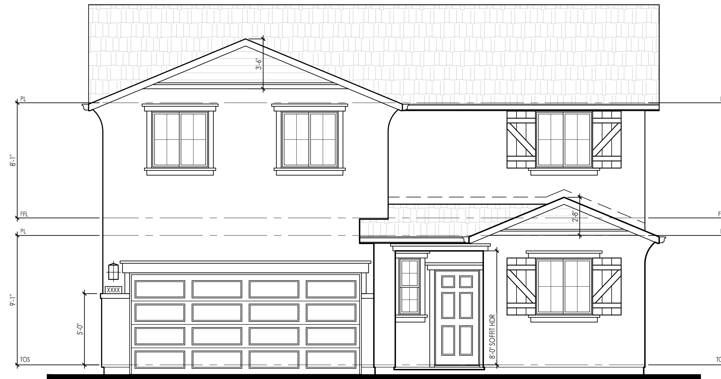
'COTTAGE' (COMPOSITION SHINGLE) FRONT ELEVATION "C" 1/4" = 1'-0"
