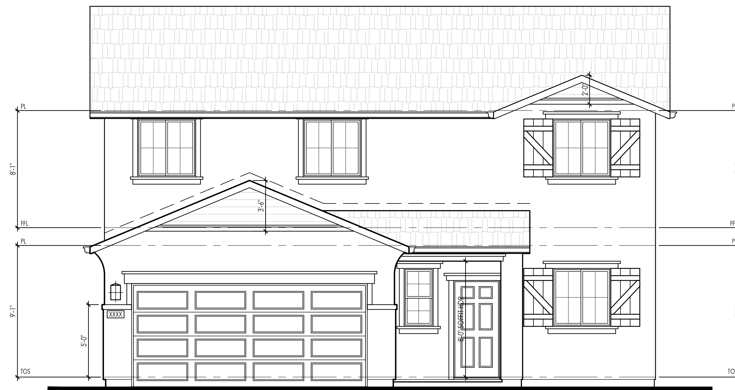
'COTTAGE' (COMPOSITION SHINGLE) FRONT ELEVATION "C" 1/4" = 1'-0"
