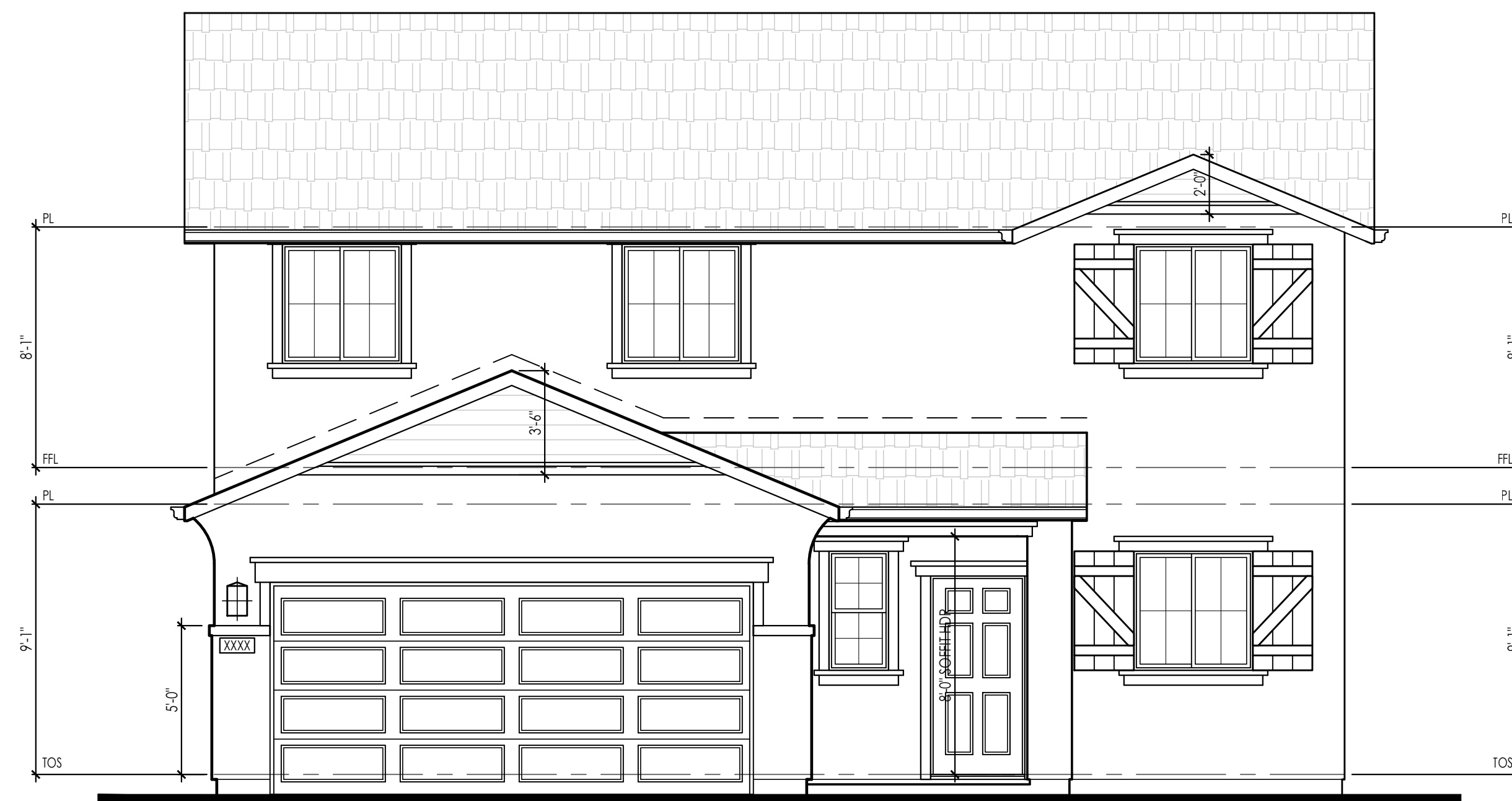
'COTTAGE' (COMPOSITION SHINGLE) FRONT ELEVATION "C" 1/4" = 1'-0"
