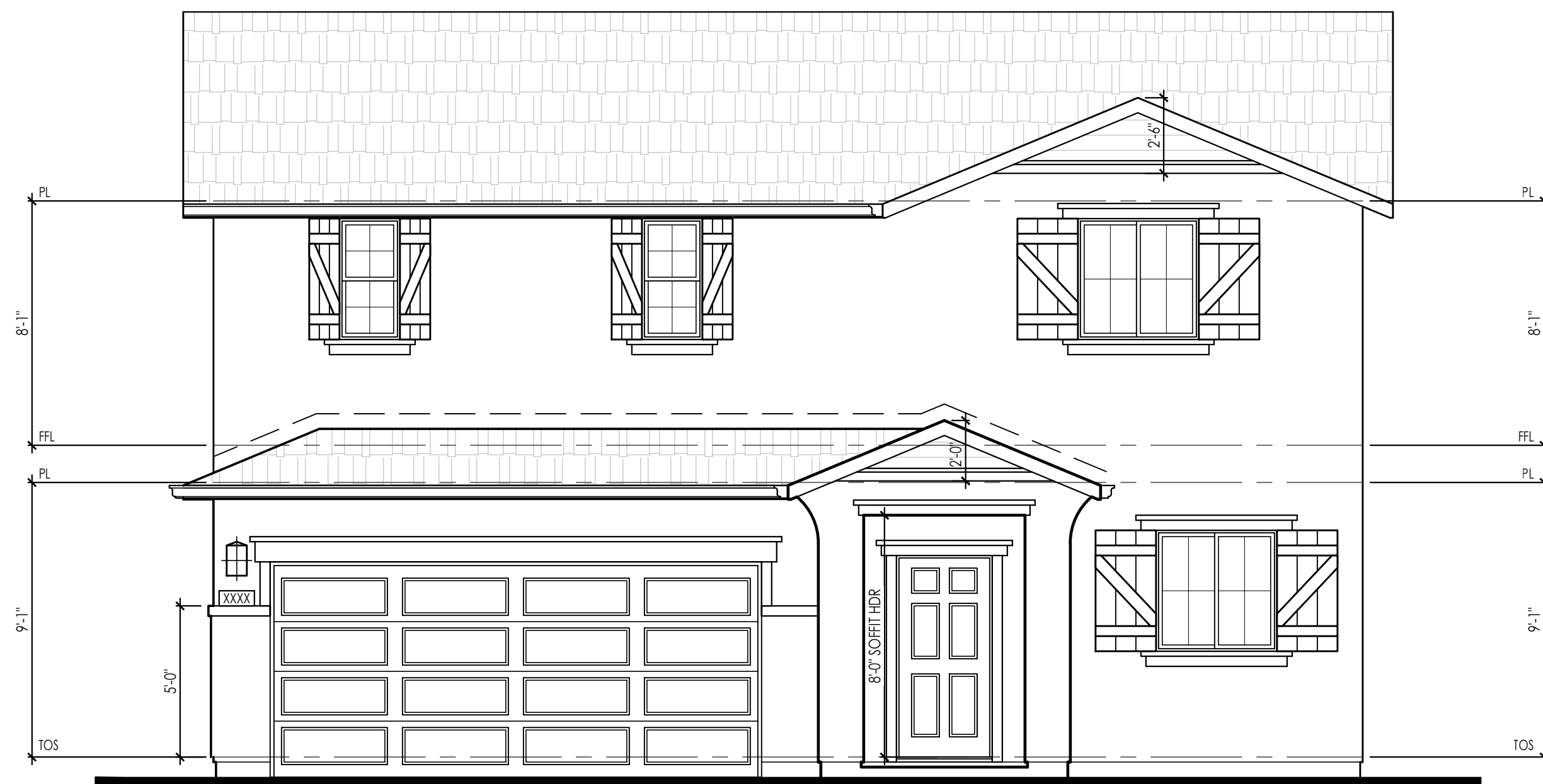
'COTTAGE' (COMPOSITION SHINGLE) FRONT ELEVATION "C" 1/4" = 1'-0"
