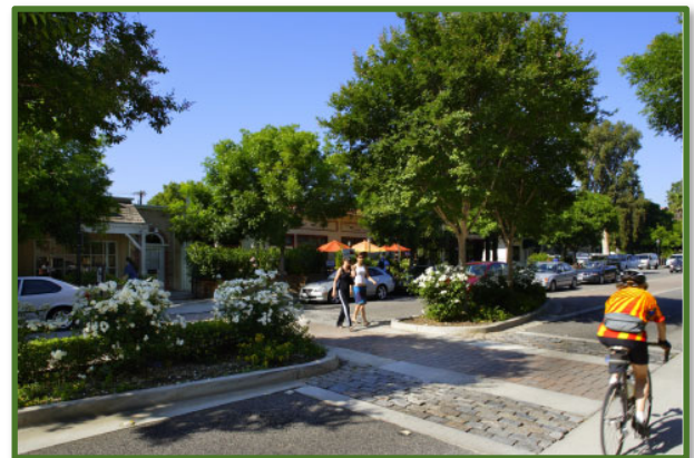
This example shows a pedestrian crosswalk with decorative paving, to help differentiate it from the road, as well as a planted median that acts as a pedestrian refuge to shorten crossing distances.
