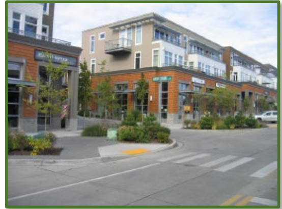
This example shows a bulb-out with landscape planting and a crosswalk; bulb-outs help slow down traffic and create shorter pedestrian crossing distances.
