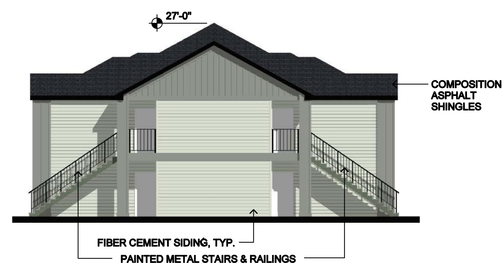
RIGHT SIDE ELEVATION BUILDING C
