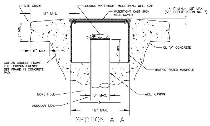
MONITORING WELL MANHOLE CONSTRUCTION DETAIL
