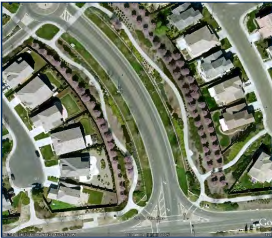
In the photo above, linear landscape areas flank both sides of a roadway. A meandering trail is located in the linear landscape area, providing a safe place for walking and bicycling that is separated from vehicle traffic.
