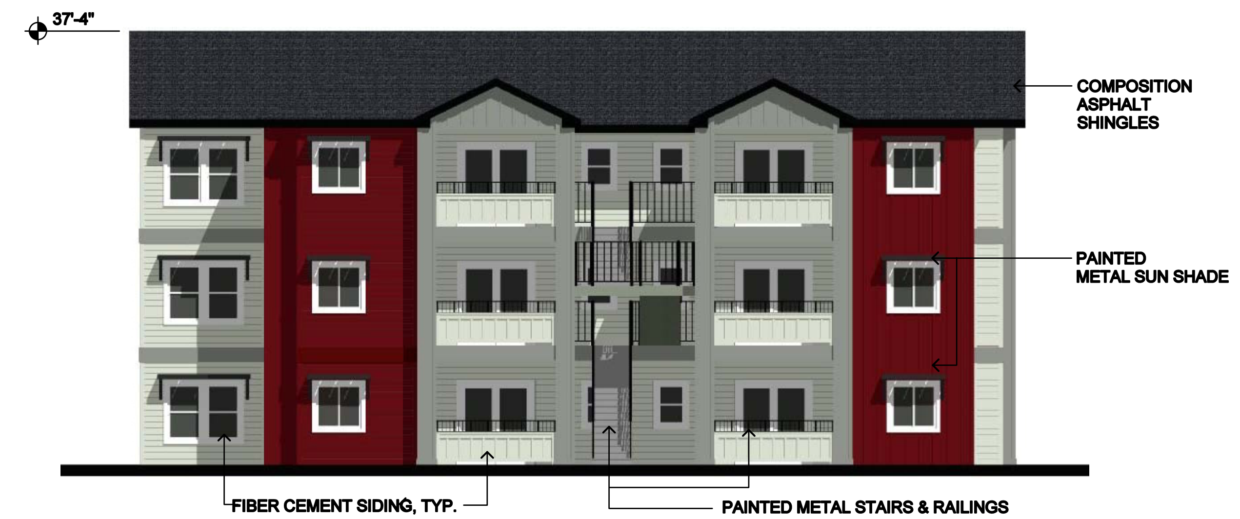
BACK ELEVATION BUILDING C
