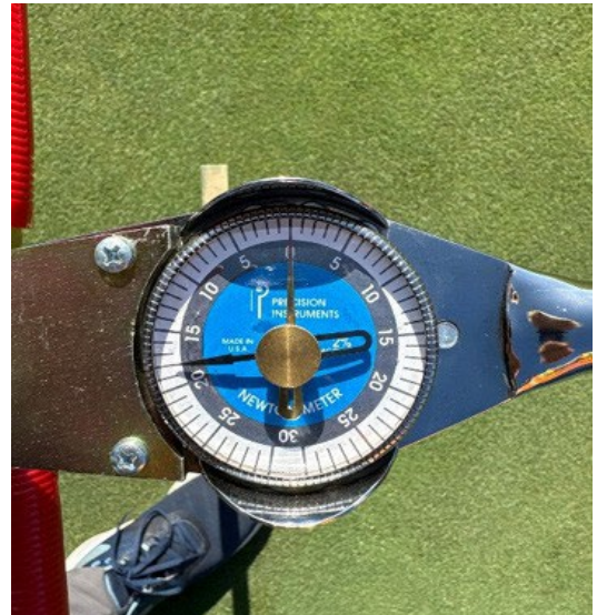
A shear strength tester was used to measure surface strength of the putting greens on hole Nos. 5 and 18. Values ranging from 16 to 18 Nm were found.
